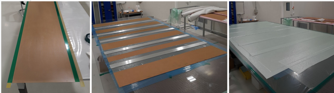
Figure 3.34. Left: preparation of PCB segment for epoxy application. Middle: six PCB segments are glued, aligned and ready to be sealed. Right: glued assembly is under vacuum for drying.
