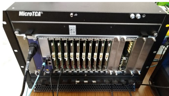
Figure 4.20. \mu TCA crate with a 40 Gbit/s MCH.
