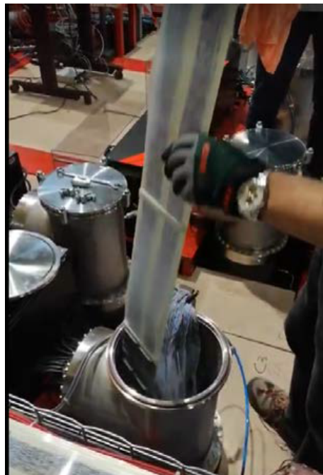
Figure 4.13. Access to a FE cryogenic amplifier card in a SFT chimney.
