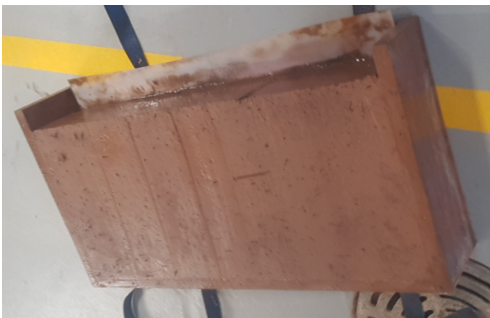
(c) Blocks removed from tank and front face trimmed
