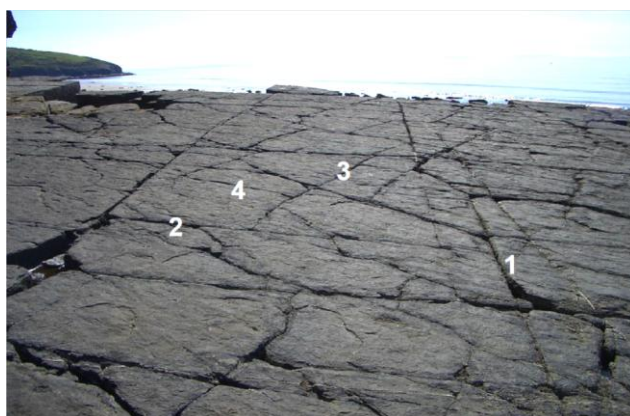
Fig. 3.16. Possible sequence of fracturing in a limestone rock mass (image courtesy of Hudson (2013))
