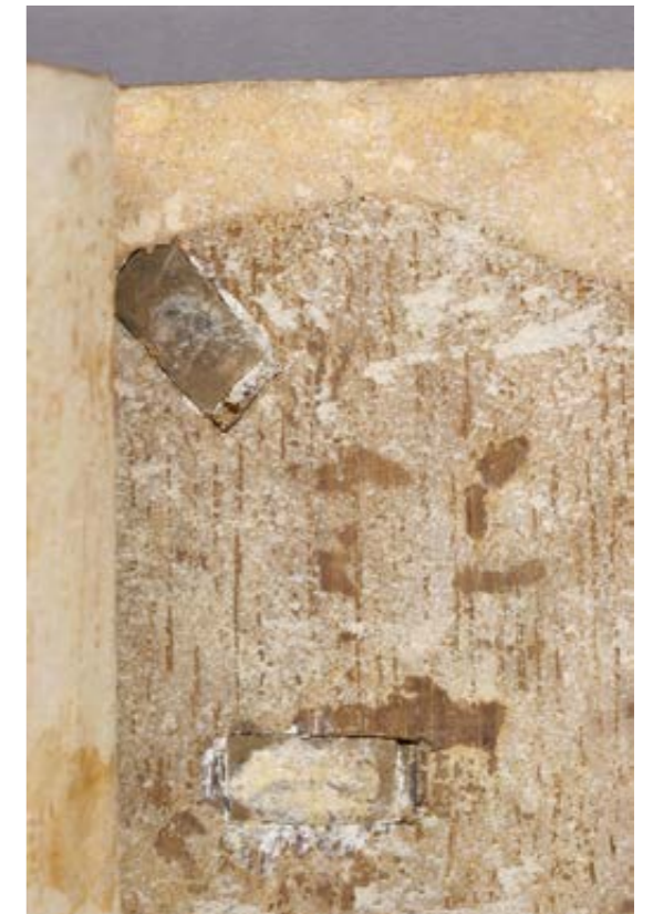
[PLATE 33] The inner face of the right board: showing the endband and sewing support lacing
