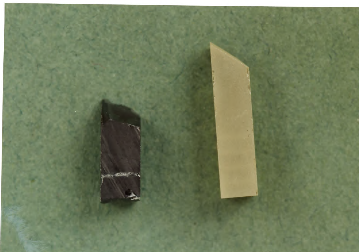
Figure 12: Stoichiometric (right) and reduced (left) examples of the single crystal rutile rods used.
