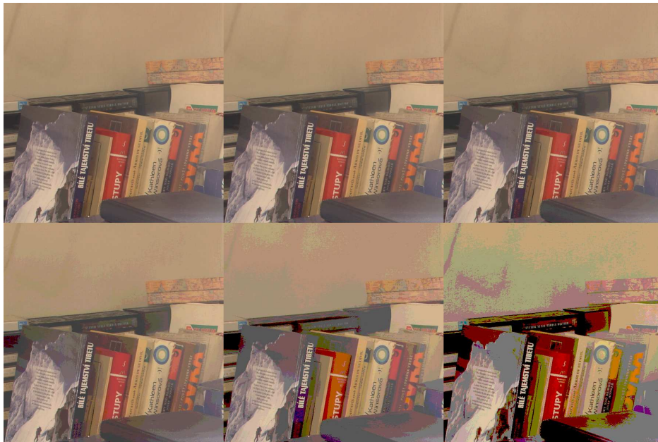
Figure 7.14: Colour quantised, cropped image of the lamp scene whose green channel has been tone mapped. The original cropped image is shown at the top left before progressively quantising it, row wise from 7 to 3 bits per colour channel.
