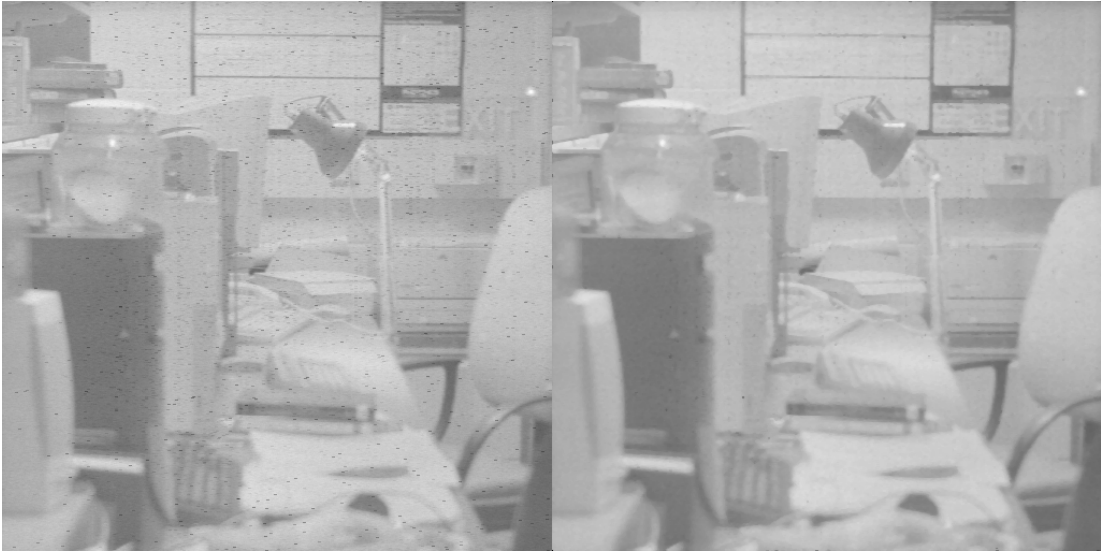
Figure 2.7: A low dynamic range indoor scene captured by the FUGA 15RGB camera and then offset corrected by subtraction of a stored image. On the right, the image is median filtered using a 3 \times 3 kernel to spatially filter off outliers.
