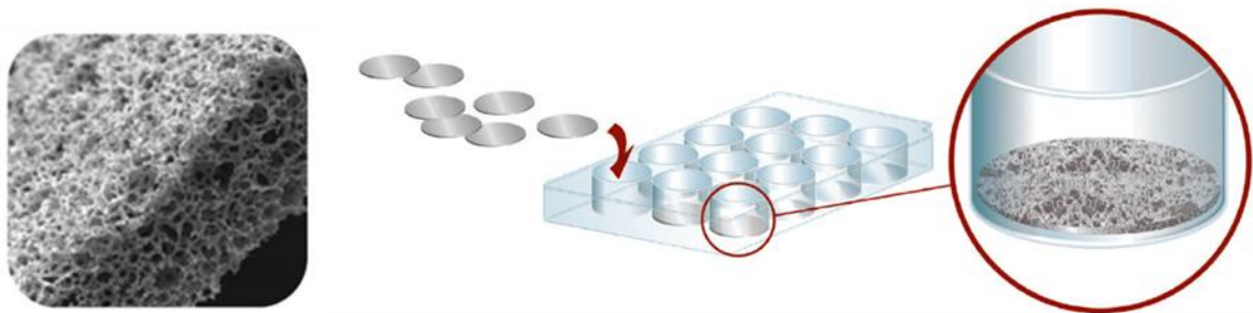
Figure 2.16: SEM of cross-section through Alvetex. Cells proliferate and fill the space created
