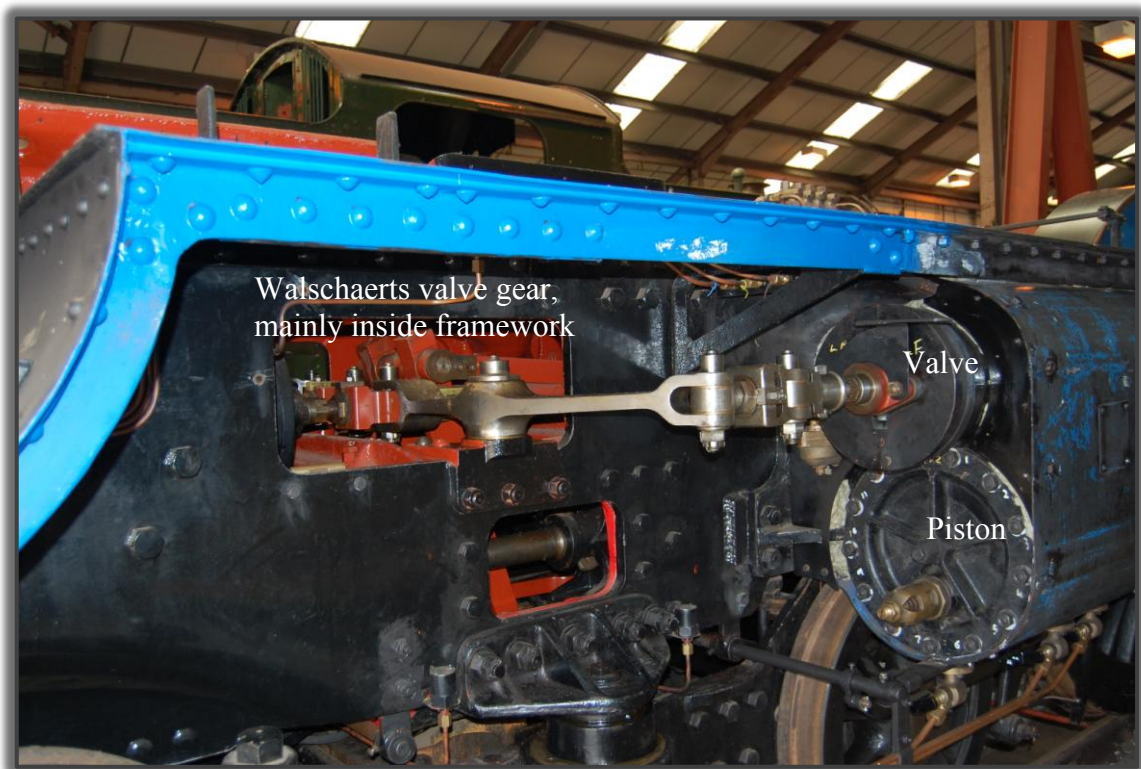
Figure 9: Timing gear on locomotive 6023
