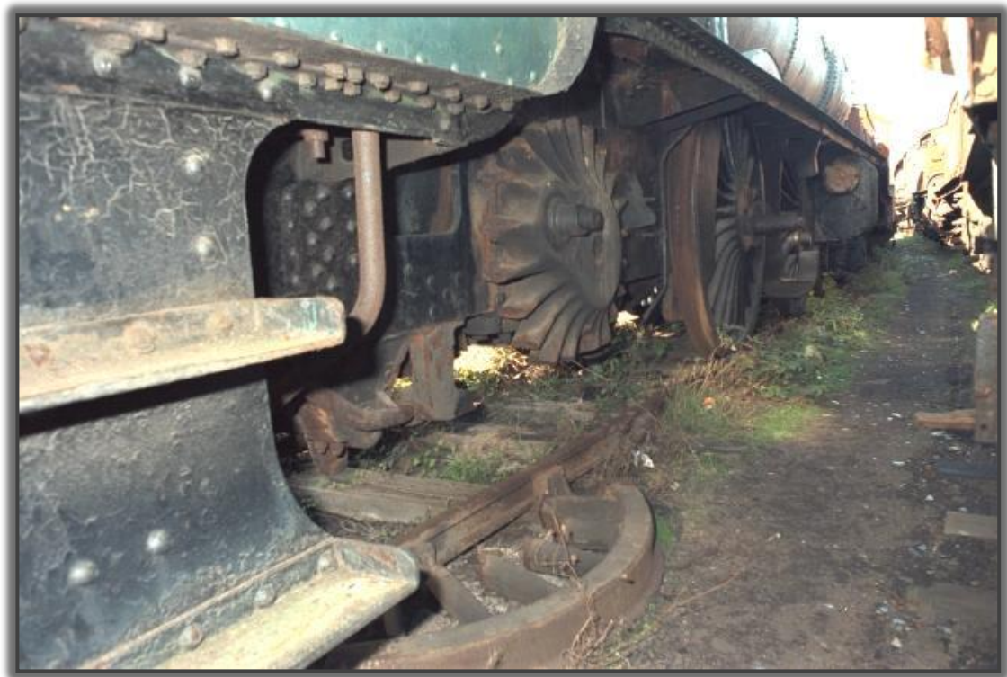
Figure 16: 'King Edward II' at the Woodham bros. scrapyard. Note the cut-away rear wheel, with discarded segment in the foreground (courtesy of Lionel Smith)
