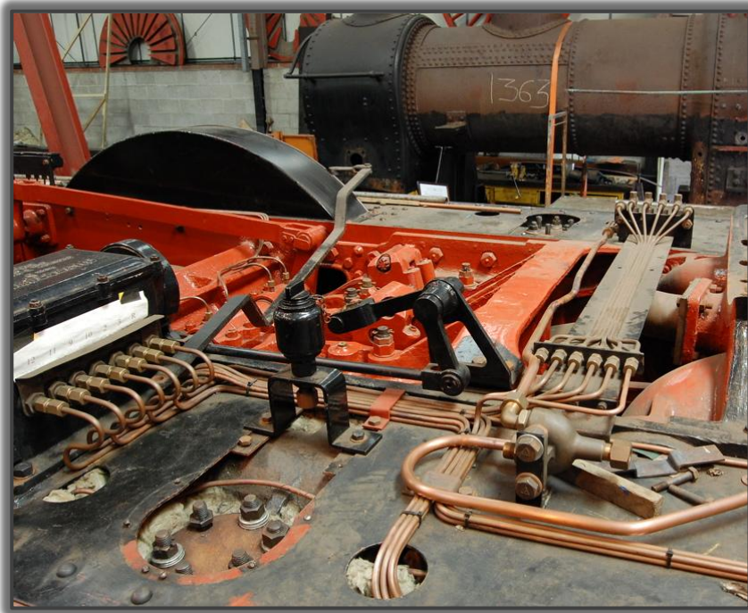
Figure 38: Part of 6023's lubrication system, made with hand-bent copper piping.
