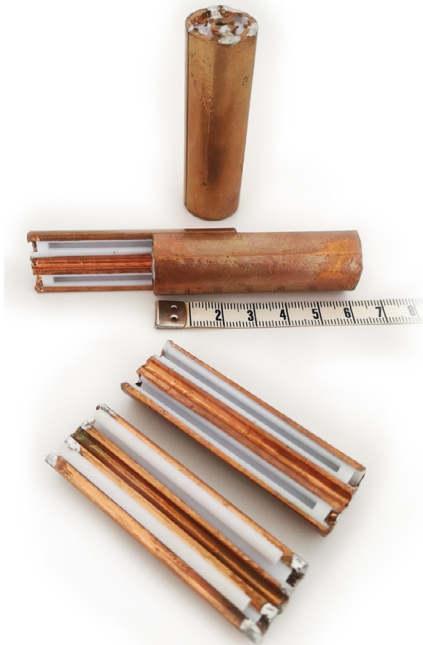
FIGURE 4 | Floating cable traps (FCTs) were built following Seeber et al. [45]. (A) Each trap featured an inner and outer conductive cylinder, separated by a Teflon dielectric cylindrical support structure and electrically connected at both ends (images show FCTs built for Site 2). FCTs measured 60 mm in length, with a diameter of 20 mm. Capacitors were embedded in the outer cylinder and were tuned to the Larmor frequency of the MRI scanner for maximum attenuation of signal propagation along the outer surface of the cable shield. (B) To protect the outer copper cylinder, each cable trap was covered with heat-shrink tubing (images show FCTs built for Site 1 and Site 3). For measurements at Site 1 and Site 3, the first FCT was placed as close as practically possible to the earpiece with the electrodes. The remaining three cable traps were spread along the cable with a 26-cm distance from each other, that is, spaced about \frac{\lambda}{10} apart. For measurements at Site 2, the first FCT was placed 32 cm from the electrodes, with the remaining traps spaced 60 cm, that is, spaced \frac{\lambda}{4} apart.
