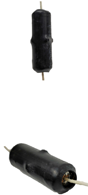
FIGURE 4 | Floating cable traps (FCTs) were built following Seeber et al. [45]. (A) Each trap featured an inner and outer conductive cylinder, separated by a Teflon dielectric cylindrical support structure and electrically connected at both ends (images show FCTs built for Site 2). FCTs measured 60 mm in length, with a diameter of 20 mm. Capacitors were embedded in the outer cylinder and were tuned to the Larmor frequency of the MRI scanner for maximum attenuation of signal propagation along the outer surface of the cable shield. (B) To protect the outer copper cylinder, each cable trap was covered with heat-shrink tubing (images show FCTs built for Site 1 and Site 3). For measurements at Site 1 and Site 3, the first FCT was placed as close as practically possible to the earpiece with the electrodes. The remaining three cable traps were spread along the cable with a 26-cm distance from each other, that is, spaced about \frac{\lambda}{10} apart. For measurements at Site 2, the first FCT was placed 32 cm from the electrodes, with the remaining traps spaced 60 cm, that is, spaced \frac{\lambda}{4} apart.
