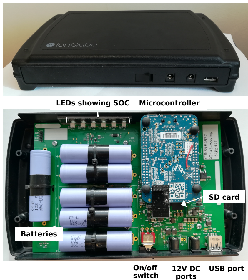
Figure 4.1: Photo of household battery in the case study, external view (top) and internal hardware (bottom).
