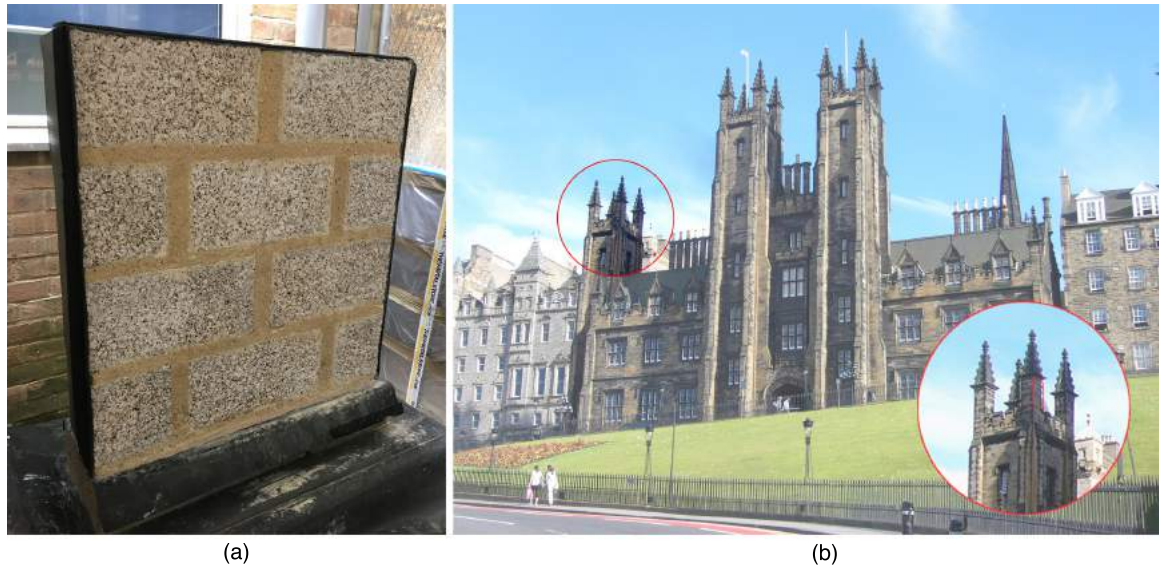
Figure 7.1. The two masonry constructions evaluated in this study. (a) The purpose built granite wall; (b) New College, Edinburgh; the area circled in red represents the tower on which evaluations were undertaken. The latter is adapted from 'New College on the Mound, Edinburgh' by Kim Traynor, Wikimedia, CC BY-SA 3.0.
