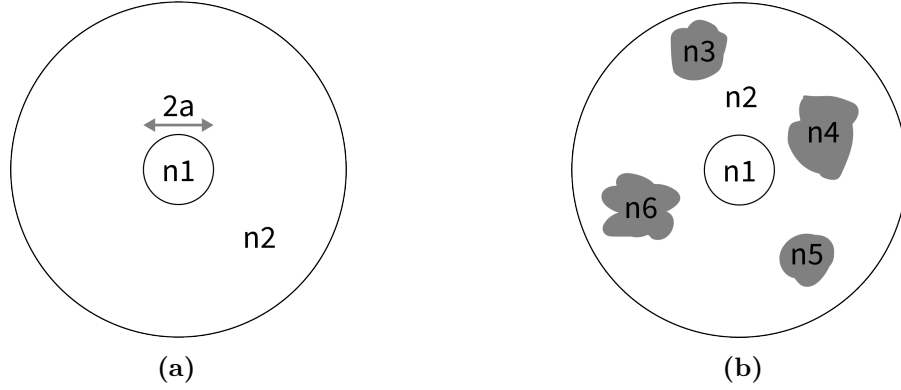
Figure 4.16: (a) Step-index Optical fibre cross sections with core radius a ; (b) General Optical fibre with arbitrary geometries as temperature control region
