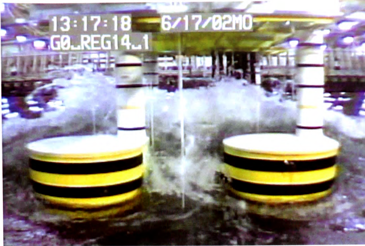
Figure 8.22: Still image showing white water beneath the LUNA model. Incident waves are propagating towards the camera.
