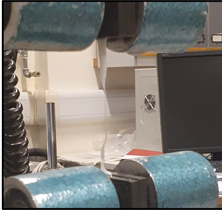
Figure 4.21: Photograph of fibre-reinforced collagen scaffold being stretched. Matrix has failed, fibre is still being loaded.
