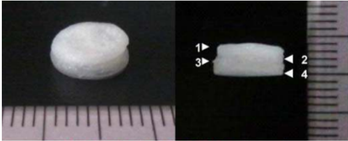
Figure 1.7: Macroscopic image of multilayer collagen-based scaffold for tendon-to-bone tissue engineering, before cell culture [114].
