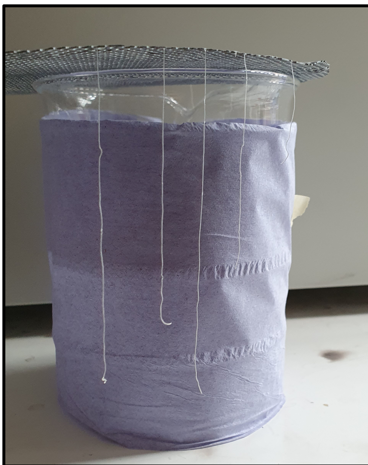
Figure 4.2: Extruded fibres air drying under their own weight.
