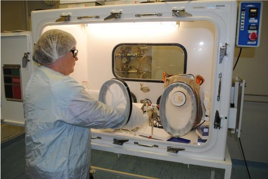
Figure 23: Class II microbiological safety cabinet used for the manufacture of S. Typhi Quailles strain at the Health Protection Agency's Porton Down GMP facility
