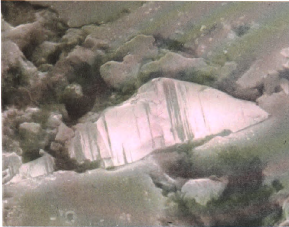
Figure 11.5. EM photograph showing an exposed particle of alumina, on the surface of a roughened femoral component.
