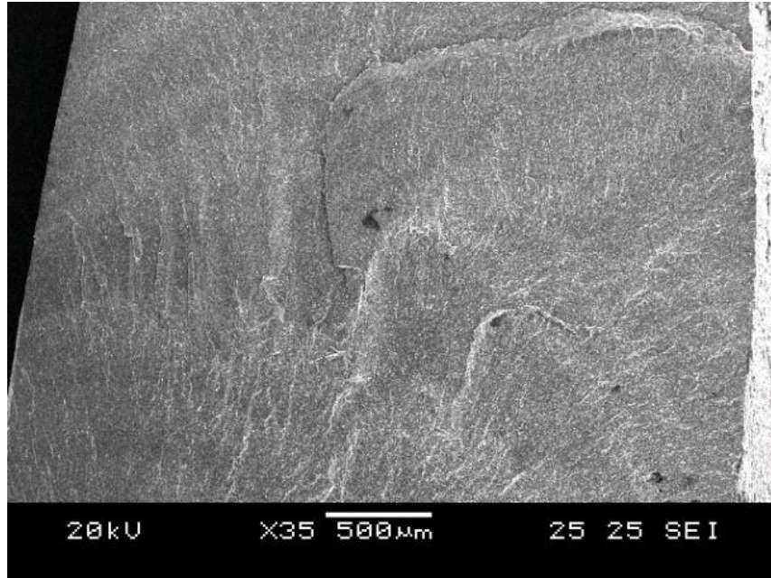
Figure 6.19: Fracture surface of the compression sample tested at room temperature
