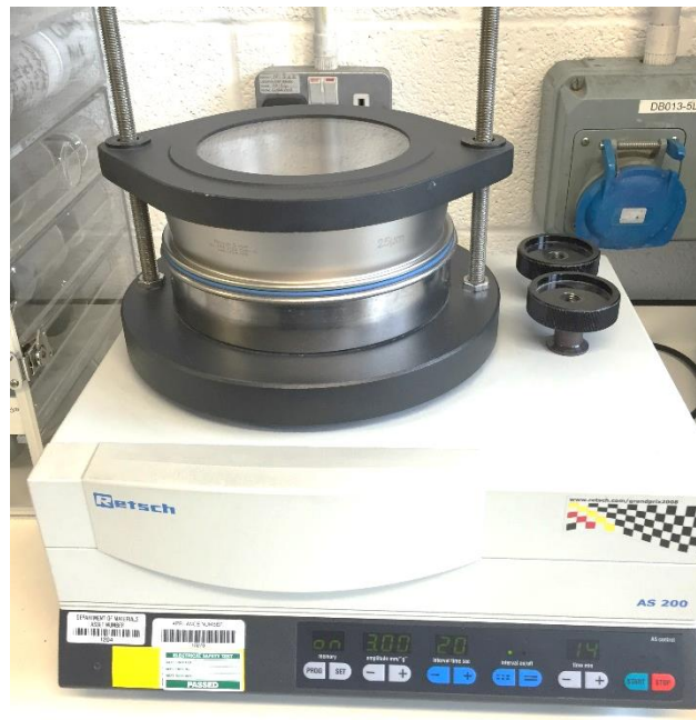
Figure 3.1: Retsch A200 automatic sieve shaker and Retsch stainless steel sieves
