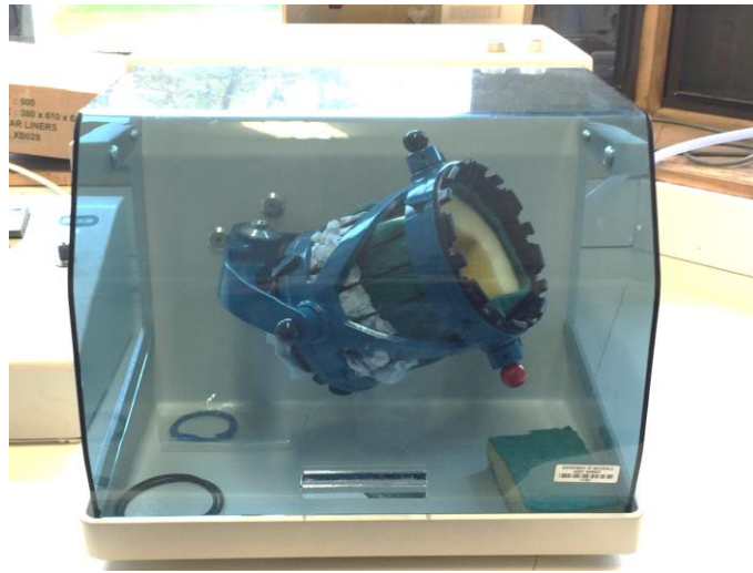
Figure 3.2: Turbula type T2F automatic mixer
