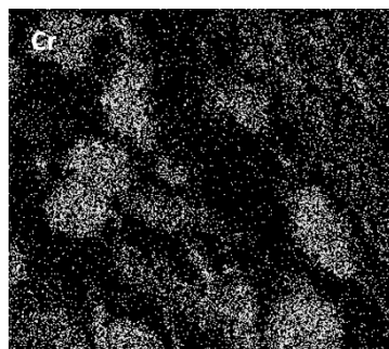
(a3) Cr EDX mapping of A250_II_5
