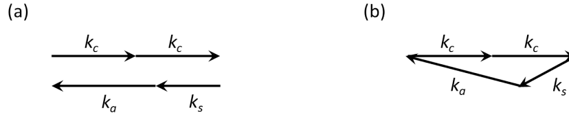
Figure 5.16: FWM phase matching condition for (a) collinear wavevectors in the absence of dispersion and (b) non-collinear Stokes and anti-Stokes wavevectors subject to dispersion.
