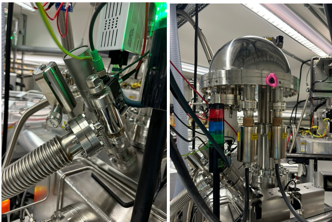
Figure 8.3 – UV-source (left) and PHOIBOS 100 analyser (right).
