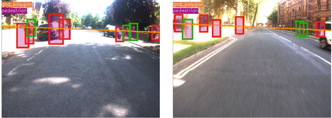
(a) Detection bounding boxes that have the bottom edge above the horizon line are rejected and stored in the memory bank.
