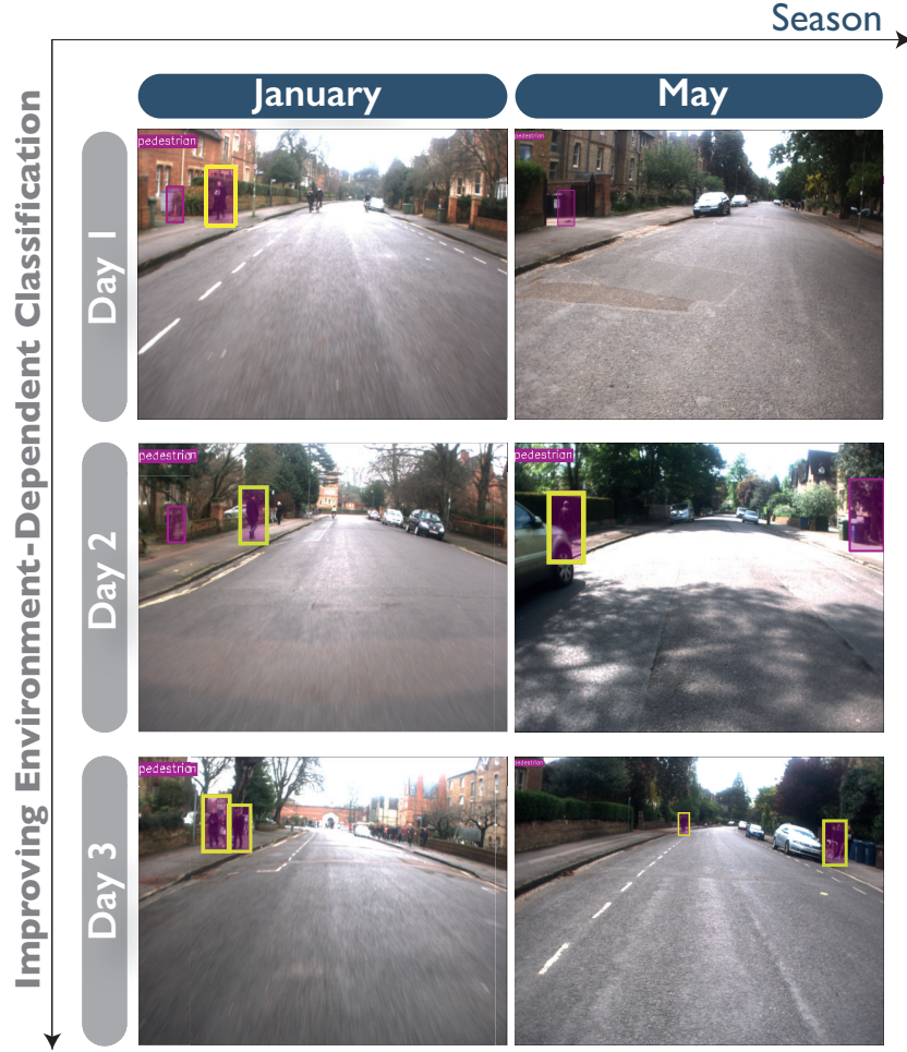
Figure 3.2: Illustration of the EBC framework: we propose detection models that learn from the robot’s experience over multiple outings. Agents are often constrained in terms of their place of operation. We take advantage of this in order to improve experience-specific performance.
