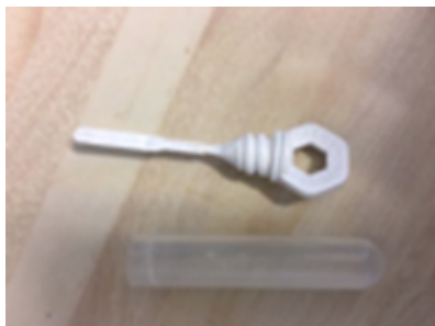
Figure 3.3 Nasosorption™ FXi nasal sampling device (NSFL-FXI-13) The SAM strip (shown) is a short strip of soft flexible fabric attached to a plastic holder which acts as a cap to its own cryotube.
