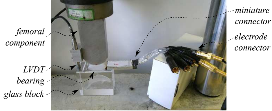
Figure 2.3: Close up of the instrumented bearing loaded with the femoral component, the LVDT compression sensor, the glass base, the miniature connector to connect the C2D to the sensor, and the electrode connector, to connect to the correct electrode. The sensors and actuator are connected to a personal computer.
