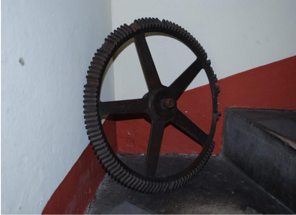
87: Model used to make cast-iron clock wheels, author, 2015.
