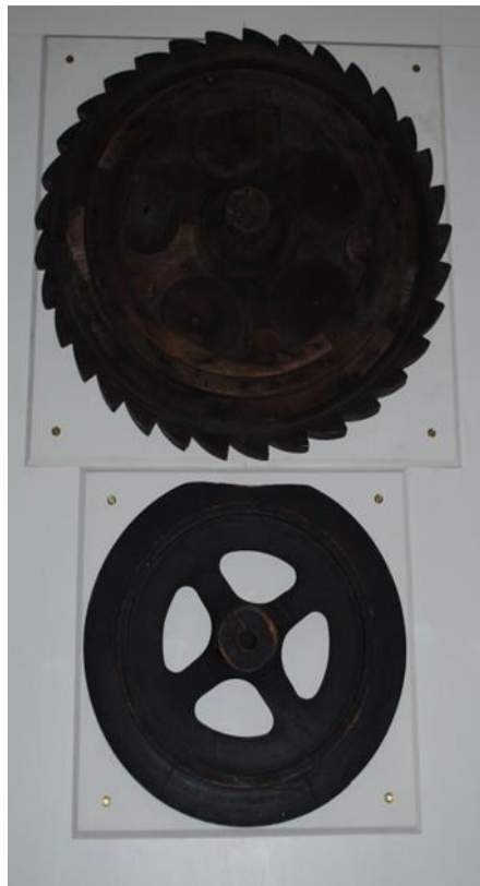
86: Wooden patterns of the clock's gears, author, 2015.
