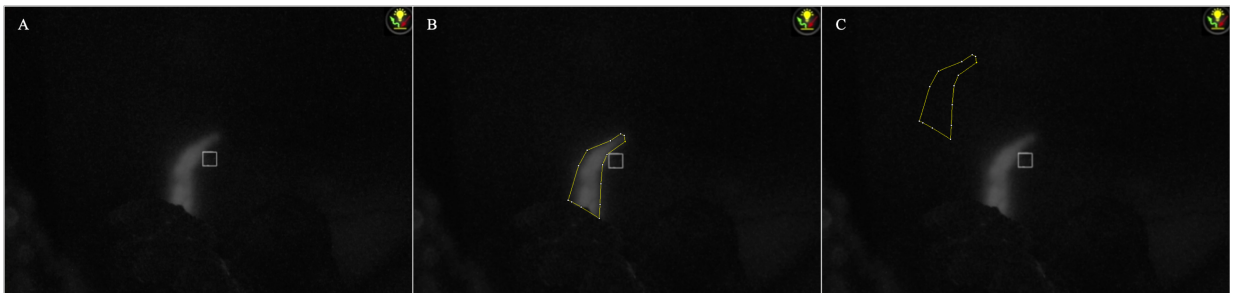
Figure 2.1 - Method of measuring signal to background ratio of NIR fluorescent image. A = image before measurement made, B = measurement of signal, C = measurement of background.
