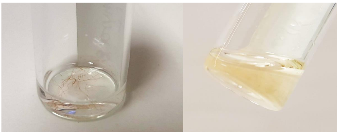
Figure 115. Before (left) and after (right) the solubilisation in 7M \text{Ca}(\text{NO}_3)_2 solution: sample S8-weft, taken after 20mins of boiling
