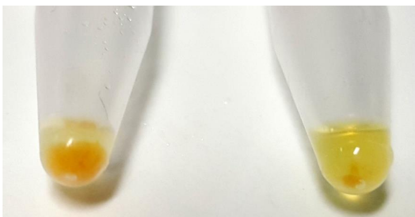
Figure 26. Re-aggregated proteins after sitting the samples for 24 hours at 4°C. left) fibre weight to solvent ratio at 1:1 right) at 1:1.5, with formic acid (1%)
