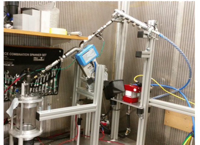
Figure 3: Experimental set up: high pressure diesel fuel line, Coriolis flowtube, injector, cylinder.
