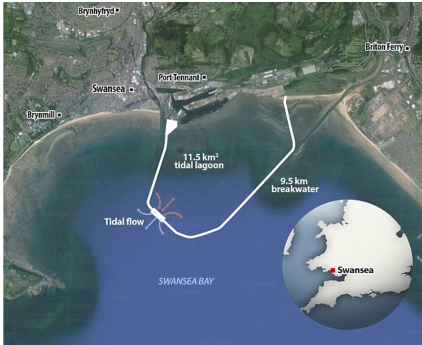
Figure 2.37: Schematic of the Swansea Bay Lagoon taken from [89].
