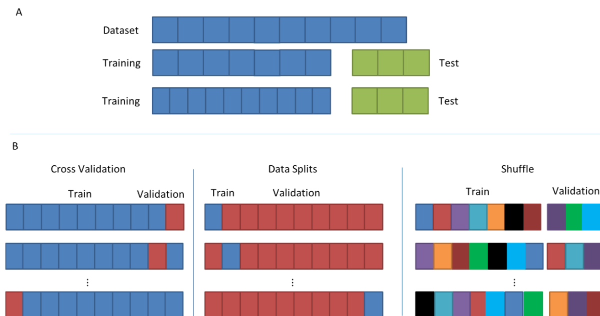
Figure 17 A) Dataset is firstly split into training and test sets either randomly or using another splitting strategy B) Training data is then divided into training and validation datasets either using cross-validation, data splitting or shuffling.
