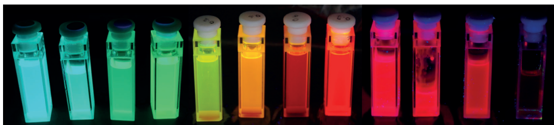
Figure 4.1: Photo of perovskite NCs made via Hot Injection synthesis under UV illumination. From Left to Right: \text{FA}_x\text{Cs}_{1-x}\text{PbBr}_3 ( x = 0.2, 0.4, 0.6, 0.8 ), \text{FA}_x\text{Cs}_{1-x}\text{PbI}_{1.5}\text{Br}_{1.5} ( x = 0.2, 0.4, 0.6, 0.8 ) and \text{FA}_x\text{Cs}_{1-x}\text{PbI}_3 ( x = 0.2, 0.4, 0.6, 0.8 )
