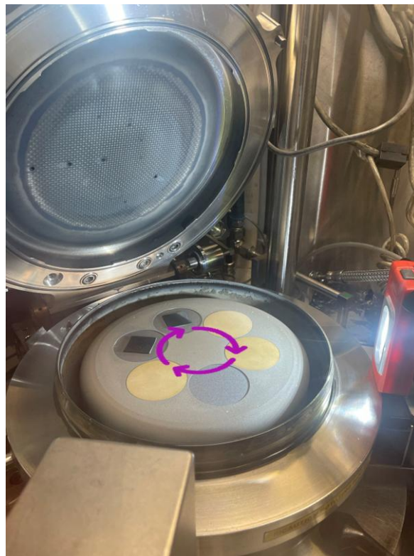
Figure 3-1 Open reaction chamber of a MOVPE reactor. The showerhead lid (top) delivers precursor gases, while the SiC-coated graphite susceptor (bottom) rotates to ensure uniform deposition on four mounted wafers and two square samples. Photograph taken on an Aixtron reactor at the Cambridge Centre for Gallium Nitride
