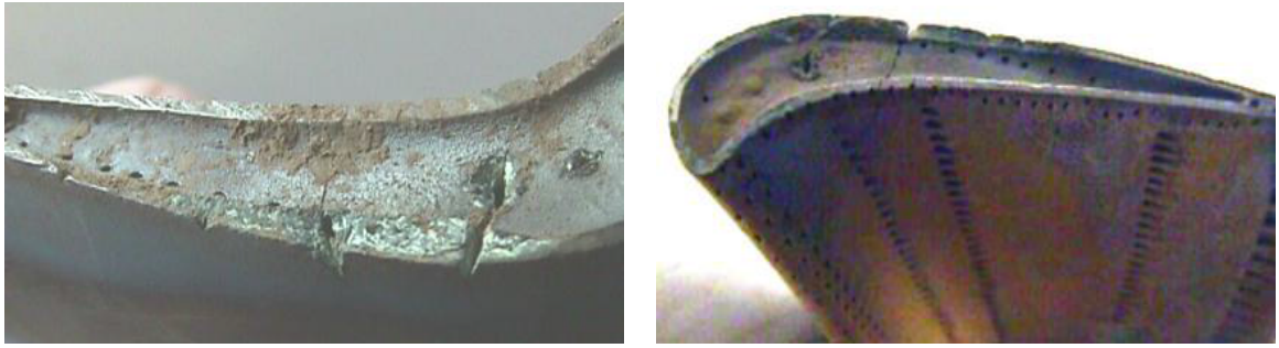
Figure 1.5: Distressed unshrouded turbine blade tips (Reproduced from Bunker (2013))
