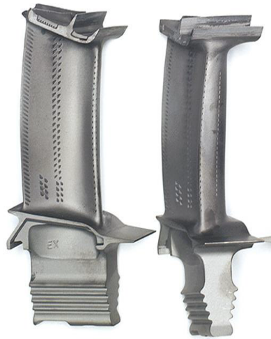
(a) Shrouded Tip: Rolls-Royce Trent 800 High-Pressure Turbine Blade After 8299 hours (cleaned)
