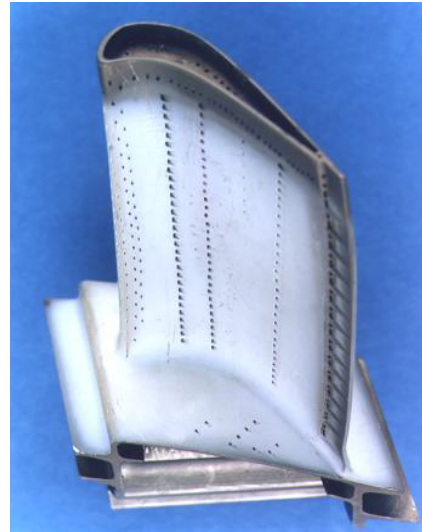
(b) Unshrouded Tip: GE High-Pressure Turbine Blade with Squealer Tip
