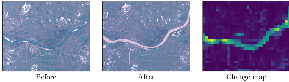
Figure 1.2: Example task with a change detection model. Having the change map predicted on-board of a satellite could be used for several triggered actions - for example sending a fast alert signal or downlinking only the relevant parts of the image (or even just the predicted mask).
