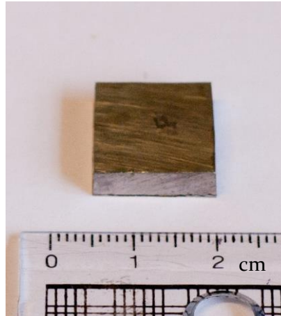
Figure 20 - Bulk EUROFER Sample slices were cut perpendicular to the flat top surface.
