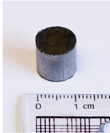
Figure 16 - Bulk Fe-14wt%Cr Sample slices were cut perpendicular to the length of the cylinder.
