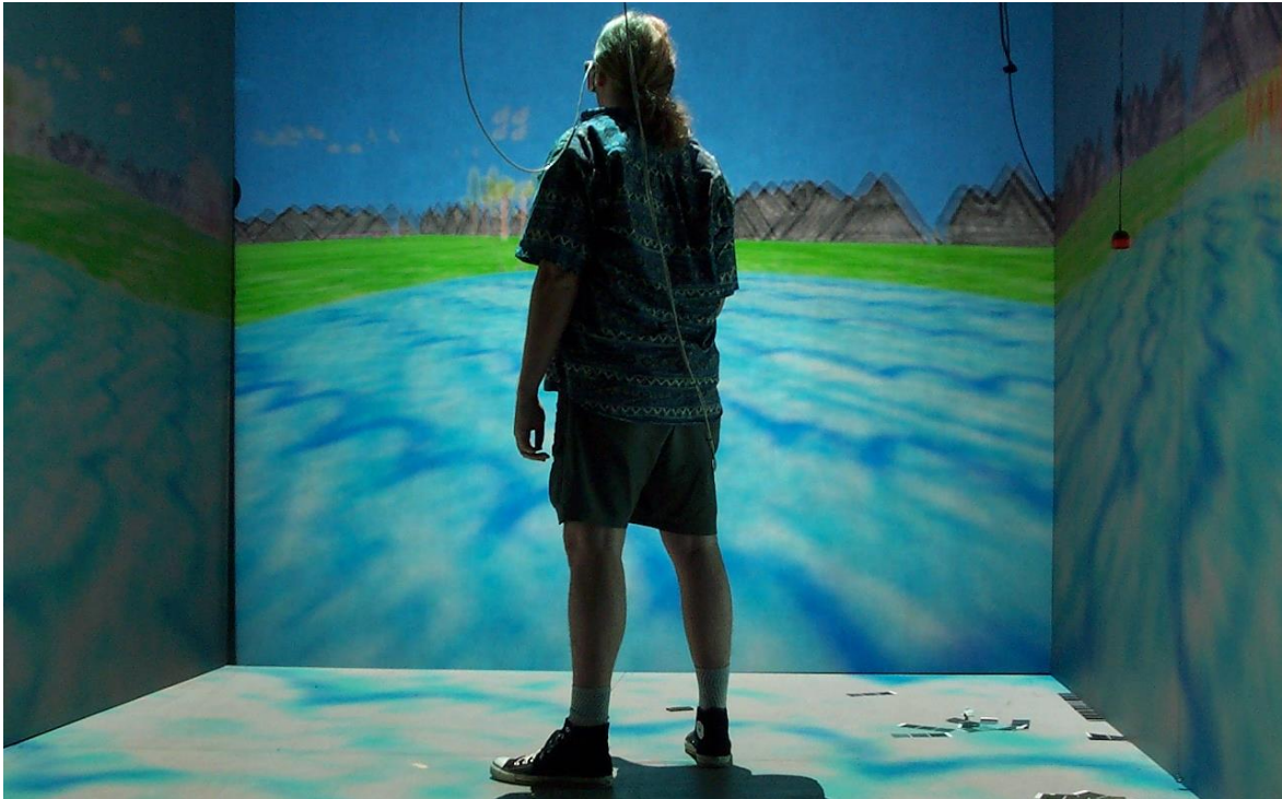
FIG. 14 A photograph of a person using a CAVE system, standing in roughly the centre of the room. Image credit: Dave Pape, Associate Professor in the Department of Media Study at the University of Buffalo. https://upload.wikimedia.org/wikipedia/commons/thumb/6/6d/CAVE_Crayoland.jpg/1024px-CAVE_Crayoland.jpg
