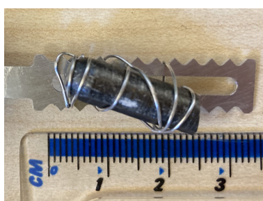
Figure 6.6: The single crystal sample of LuCoSiIG used for inelastic neutron scattering measurements. The [1 \ -1 \ 0] axis is approximately parallel to the ruler.
