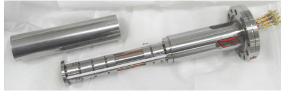
Figure 4.6: Photograph of the electron gun assembly. The mu-metal tube for magnetic shielding (top left) has been removed so that the different electrostatic lenses can be seen.
