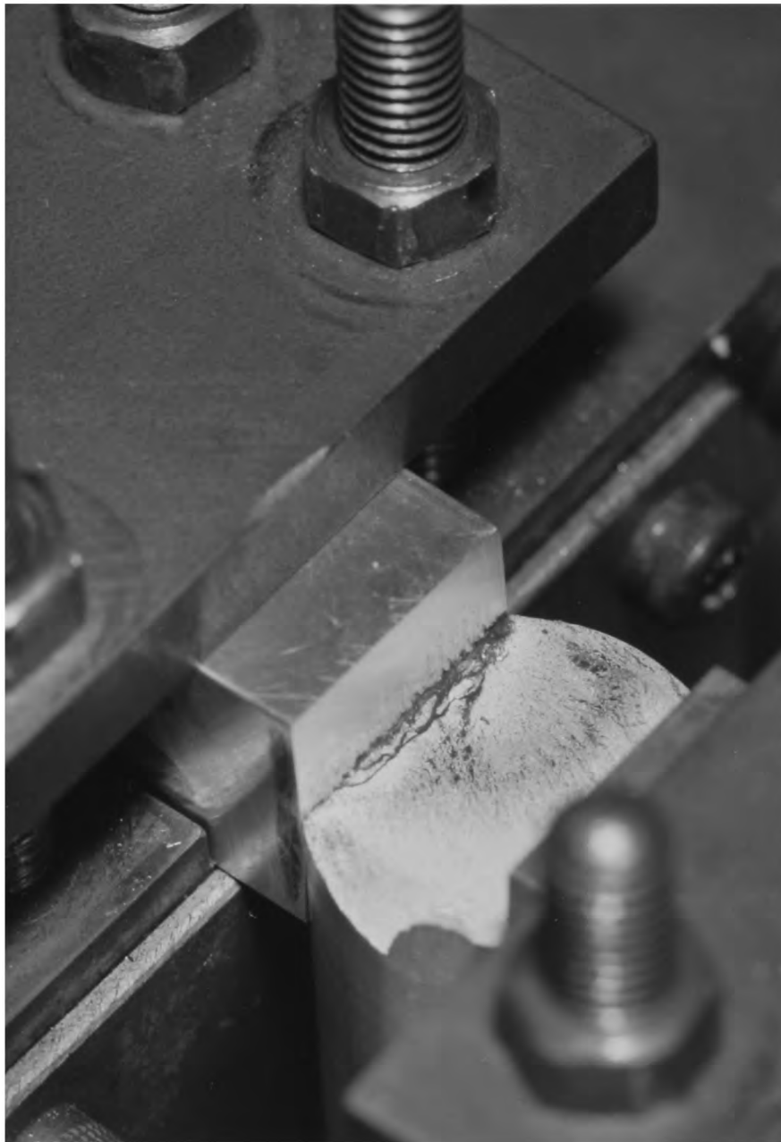
Fig. 3.2a Failed specimen in the fatigue machine
