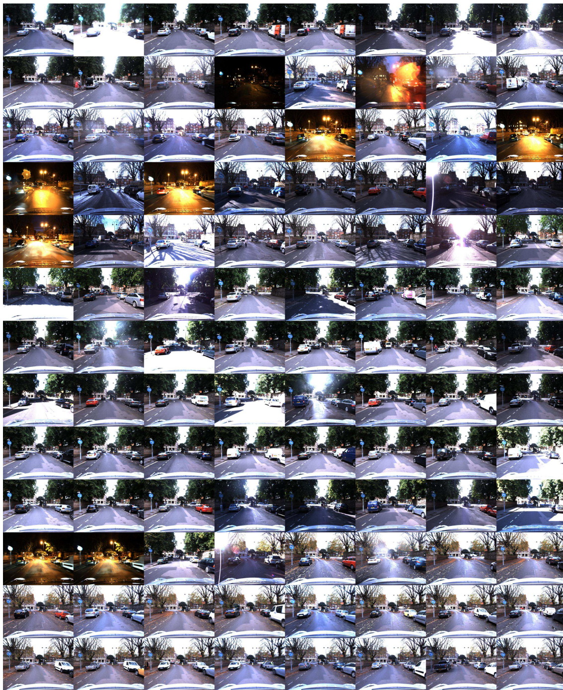
Figure 1.1: This figure demonstrates the challenge of performing robust vision-only localisation in outdoor environments. Each image in the montage is a snapshot from the same place as the robot traversed a single lap of the Oxford 10 km route (note that the blue sign post is visible in all images). The appearance of the scene is subject to sudden and unpredictable changes due to varying lighting, weather and seasonal conditions.
