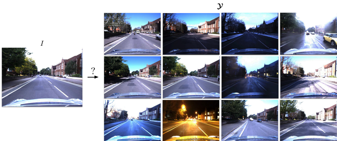
Figure 5.1: This figure illustrates the problem of experience density. The localiser queries the experience graph \mathcal{G} for the candidate nodes \mathcal{Y} nearby the robot which may result in successful localisation. As more experiences are added to the map, the number of candidate nodes increases. Given that each experience is visually distinct, the live image I may only localise in a small subset of these nodes. This chapter presents a method for ranking the candidate nodes based on their probability of localising with the live image I .
