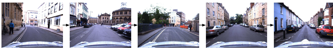
Figure 2.9: A simple map of the environment can be created by recording images as the robot traverses the environment. Visual odometry determines the motion between images, giving the map a topometric structure. At run-time, the localiser attempts to match the live image against one of the images in the map.
