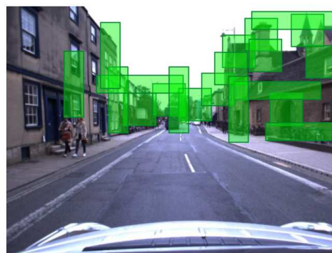
(h) This procedure is repeated for different patch sizes. Different classifier sizes result in different combinations of scene elements being used for localisation.
