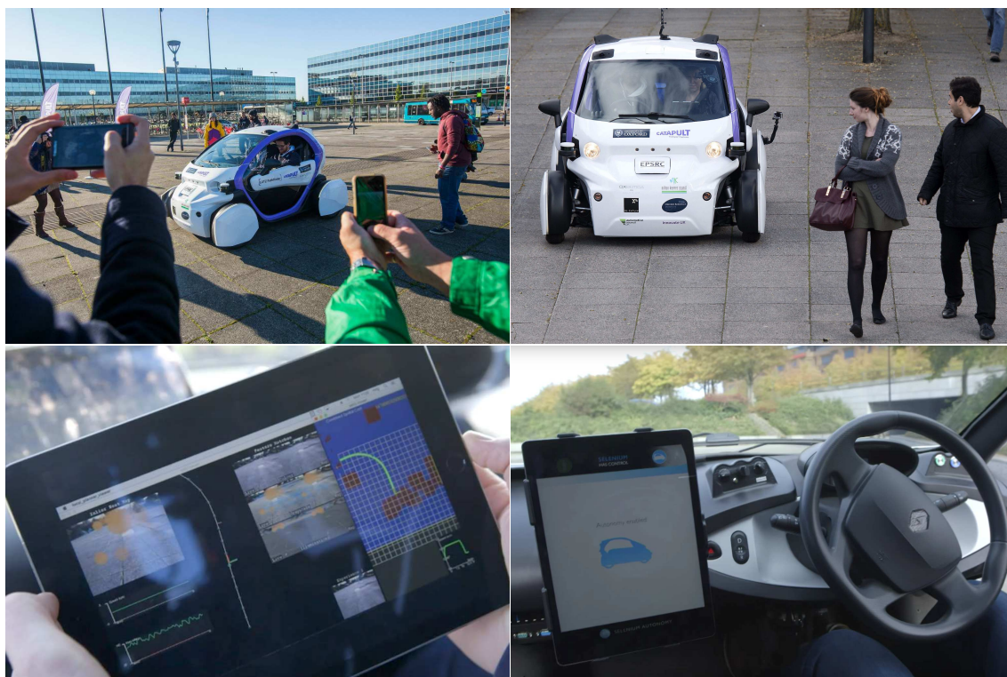
Figure 1.2: Photos of the LUTZ PathFinder trials which took place along pedestrian walkways in Milton Keynes. Dub4, the vision-only localiser described in this thesis, was used to localise the vehicle for the duration of this week-long trial.
