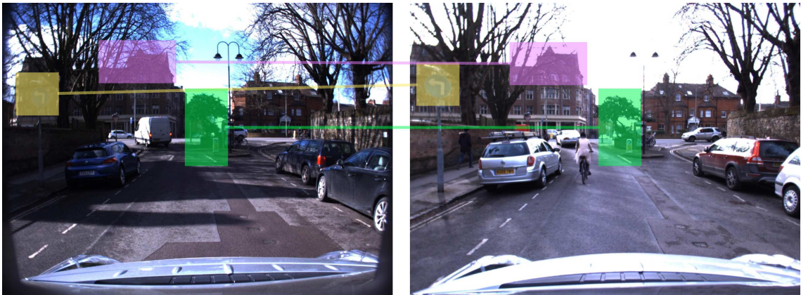
Figure 6.1: Robust landmarks in this scene might include the signpost (yellow), the tree in the intersection (green), or the building’s roof (pink). These landmarks are used to perform robust localisation across challenging appearance change in the environment.
