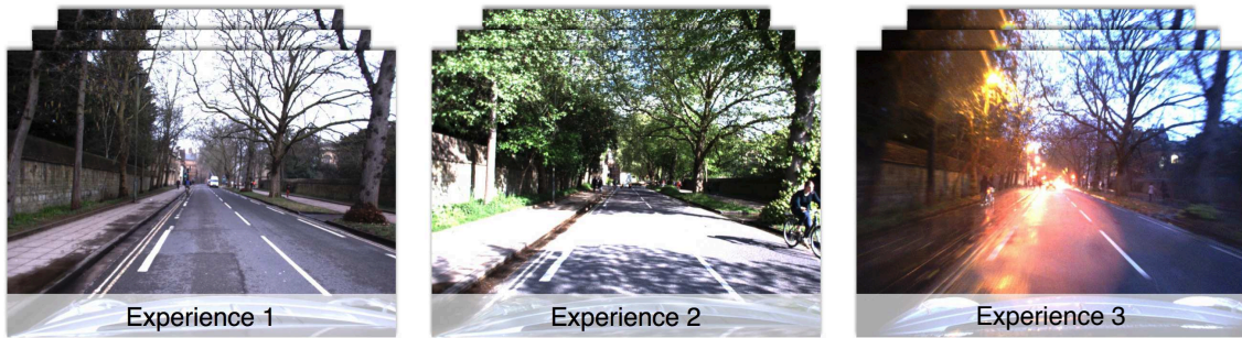
Figure 4.1: An experience is a stream of images recorded as the robot drives through the environment under particular conditions. Multiple experiences model the appearance of the world under different conditions. Three experiences are shown here, (i) a cloudy, winter’s day, (ii) a sunny summer’s day, and (iii) a rainy winter’s evening. Note that the underlying cause of appearance change is not important, but only that the appearance of the environment has changed.
