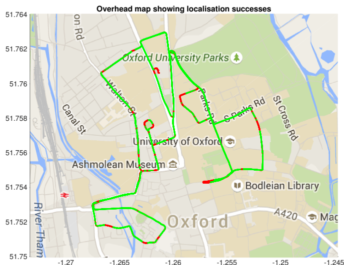
Figure 6.9: The output from a single localisation run, where a sunny log was used to create a map and a cloudy log was used to localise in the map. The trajectory is plotted on an overhead map, and the success or failure of the localisation attempts are plotted in green and red, respectively.
