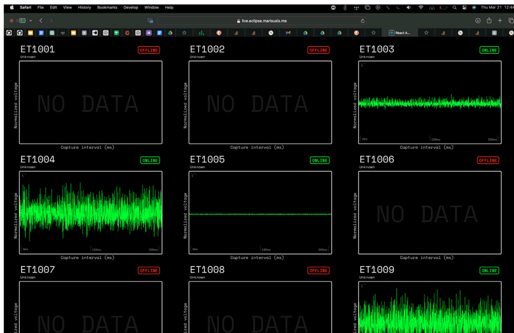
FIGURE 5 Screenshot of the web dashboard built for remote, real-time monitoring of the ET unit data collection.
