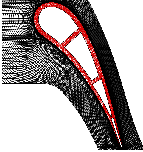
Figure 4.5: Mesh used for the conjugate solution.
