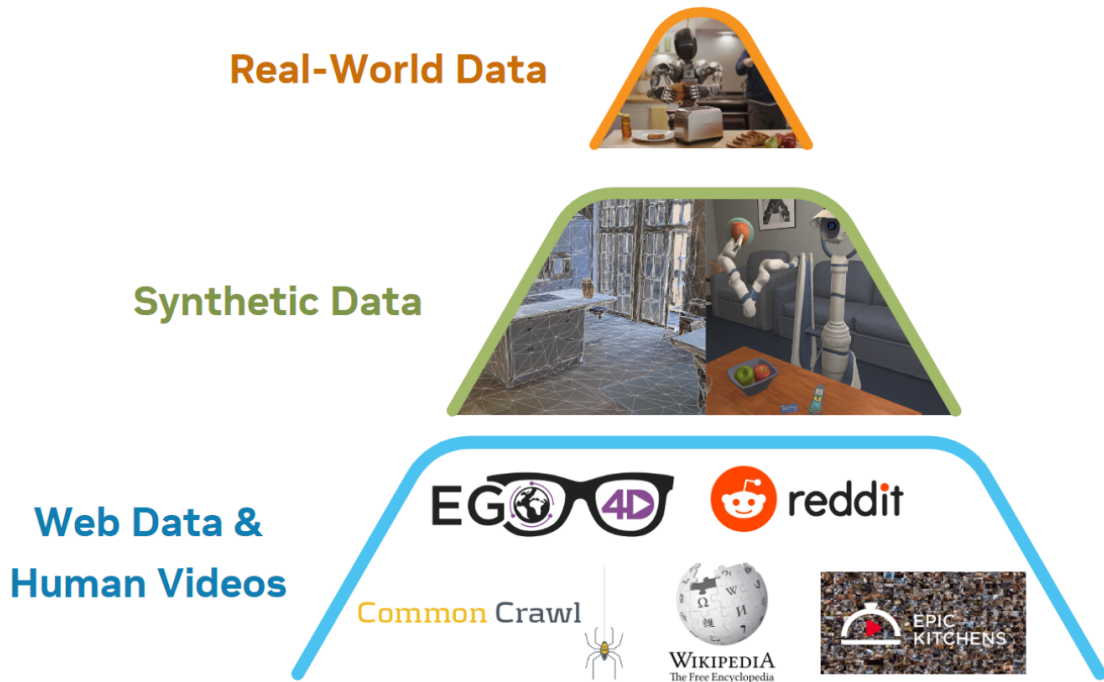
Figure 5.3: Data pyramid of different data sources for training generalist robots. The data quantity decreases from bottom to top, while the data quality, i.e., alignment with the target robot in embodiment, task and environment, increases. Image credit to NVIDIA et al. [2025] .
