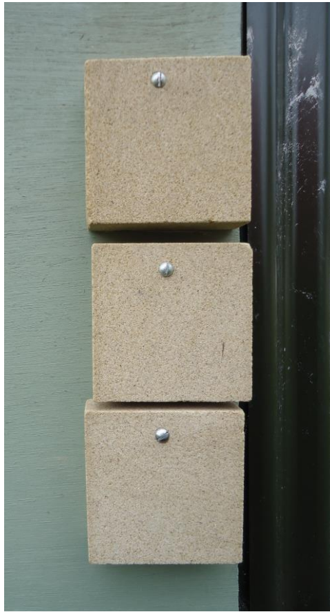
Figure 41: Dungannon samples exposed vertically on test structure
