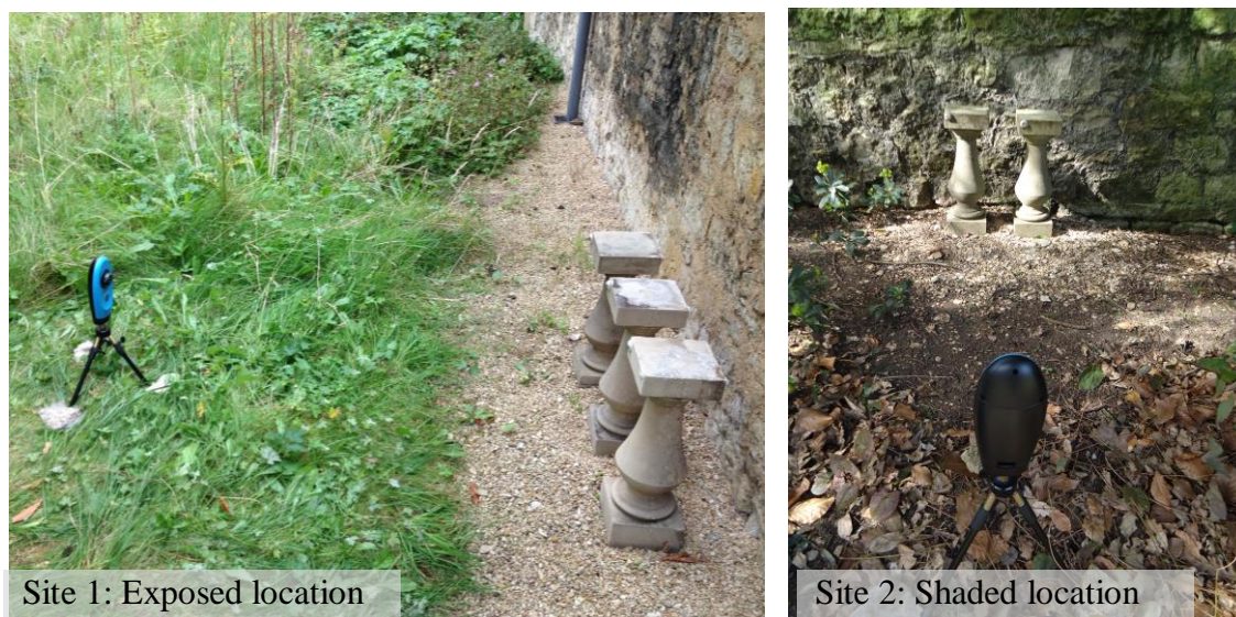
Figure 98: Time Lapse Camera (TLC) set-up at both field sites
