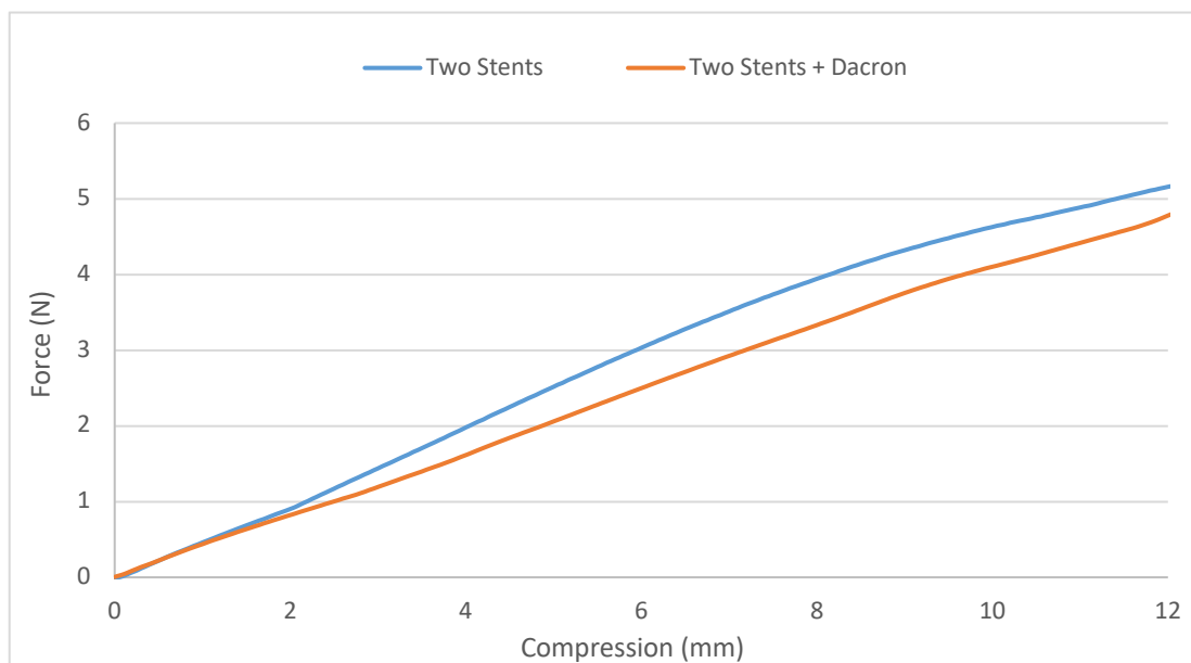
Figure 4.35 – Comparison of flat plate compression forces between two stents and two stents stitched to Dacron fabric. Stents all have a wire diameter of 0.44mm.
