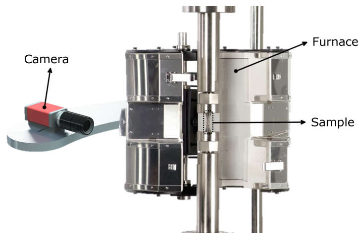
Figure 3.1: The Instron TMF test bench with furnace and camera installed.
