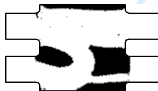
Figure 16: Optimised topology for the double pipe joint case (Source: Authors own work).
