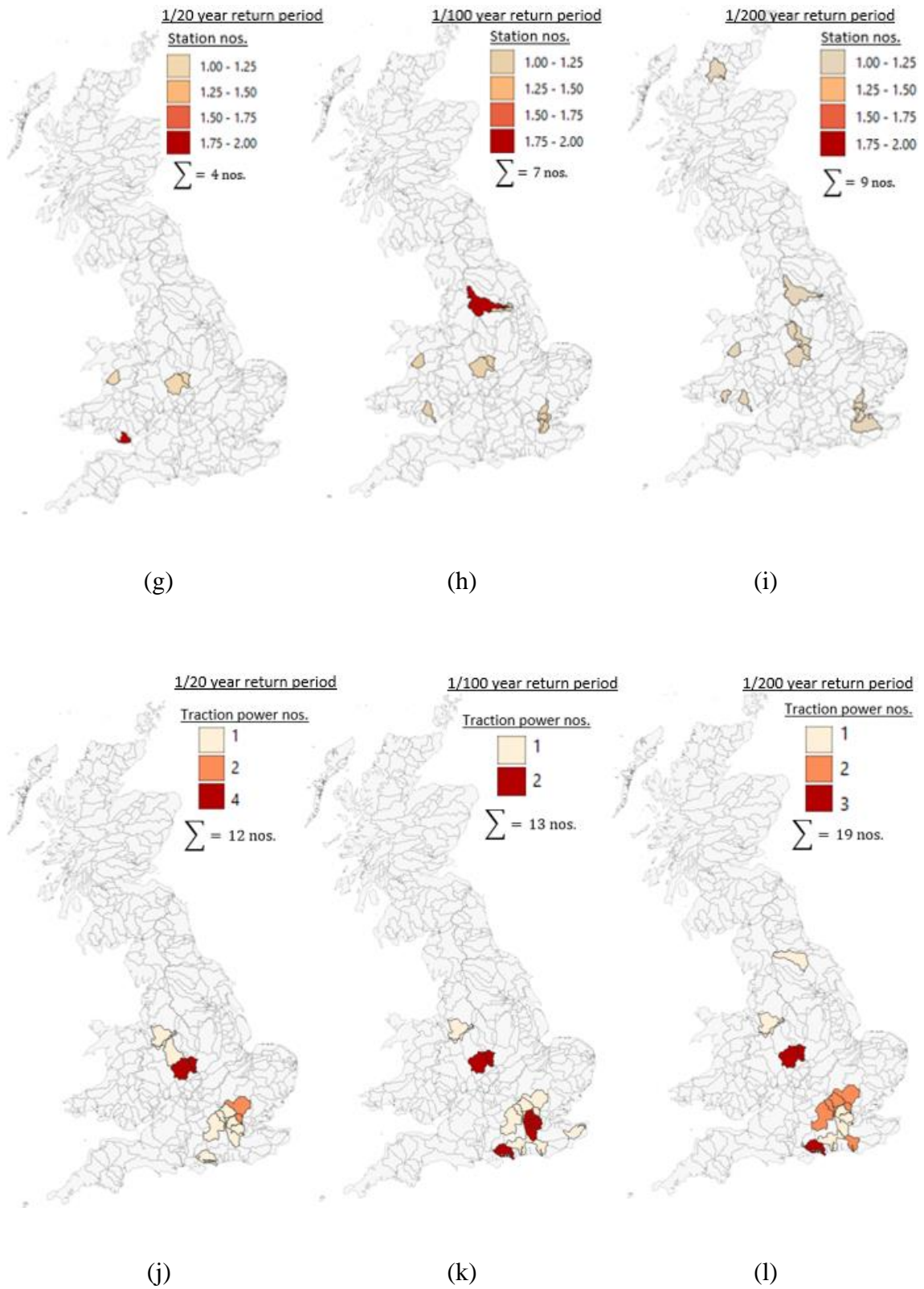
Figure 6.6 (a-l) Spatial plot of exposure analysis for rail assets for all three river flood return periods.
