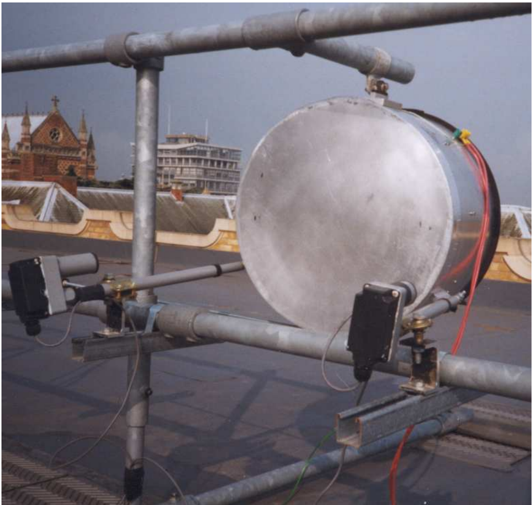
Figure 2.13: Back of external source as installed on the roof of the atmospheric physics department, showing the actuators used to control its aspect.
