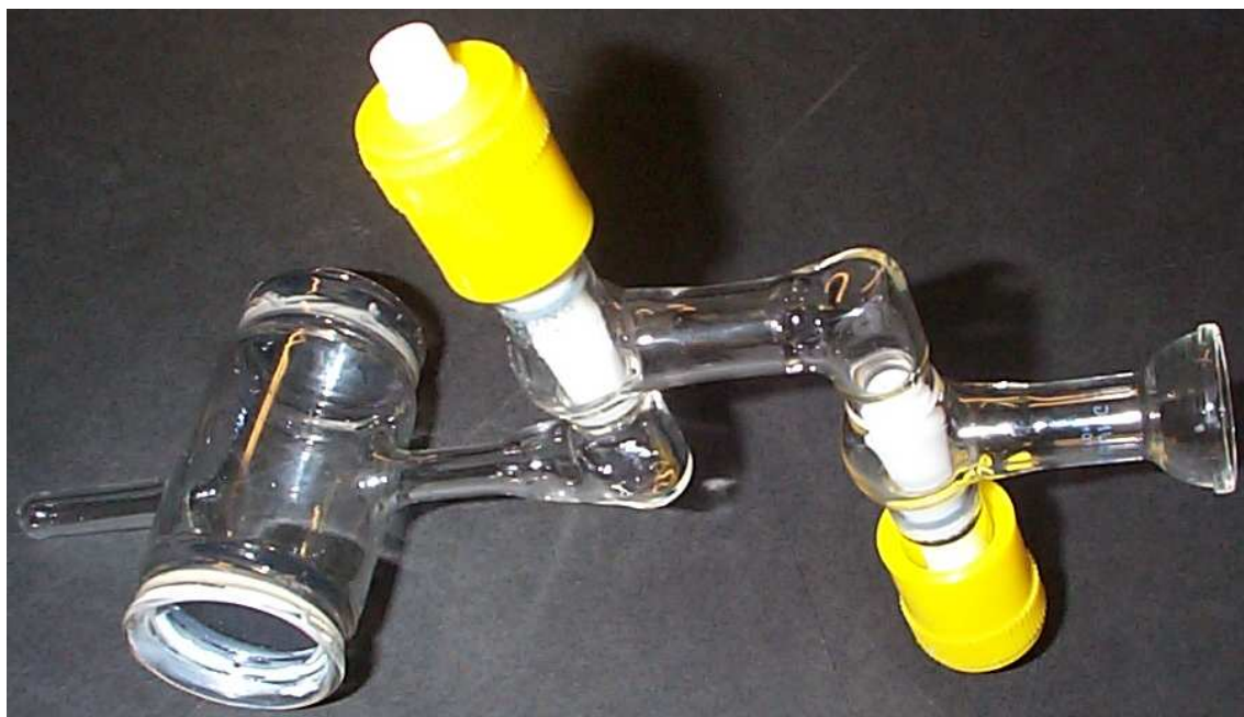
Figure 4.2: The 50.6 mm pathlength low pressure gas cell used to measure the ILS of the Perkin-Elmer Spectrum 2000 FTIR spectrometer.
