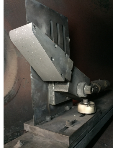
(b) The model in the test section with the blunt leading edge installed.
