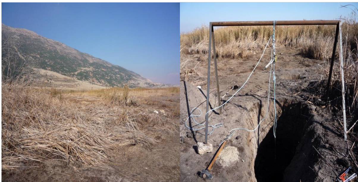
Figure 3.1 Photographs of the core site with Lebanon Mountains in the foreground, excavation of sediment around core site to facilitate extraction, and A-frame and winch.
